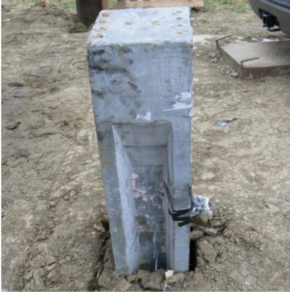
Figure 5.36. Condition of pile P2 at the end of the lateral load test
