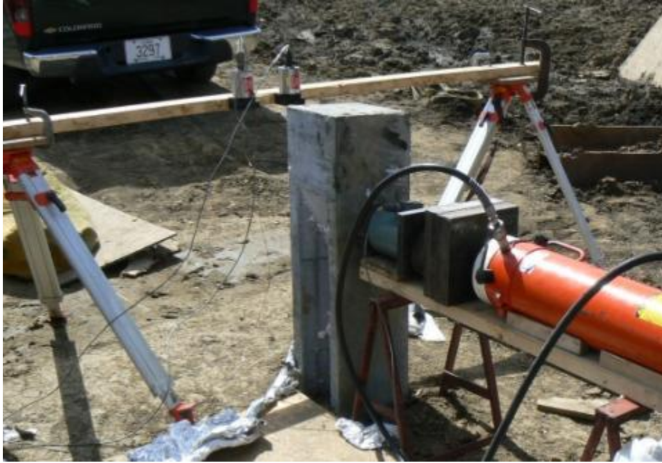
Figure 5.30. Displacement transducers attached to a wooden reference beam supported on tripods
