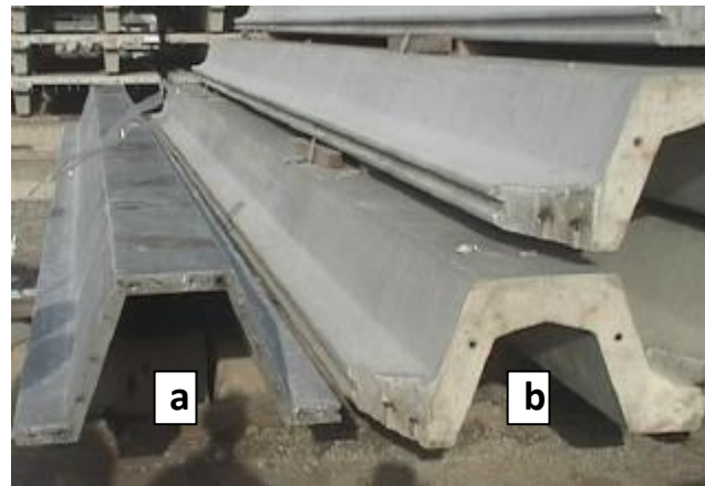
Figure 2.43. Comparison of a) SCFRC and b) conventional concrete sheet piles (Grünwald 2004)
