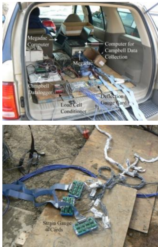
Figure 5.32. Data collection system used during the lateral load test
