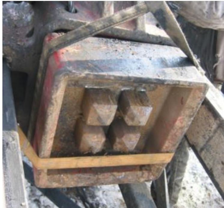
Figure 5.5. Driving helmet with guiding spikes used for steel piles
