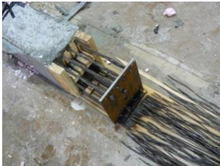
Figure 4.15. Strands released at end of UHPC pile P2
